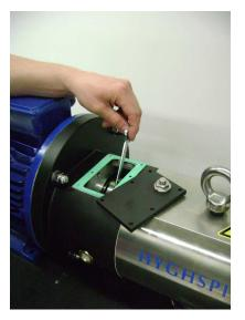
The new maintenance access opening facilitates the adjustmentof the clearance between the feed screws
