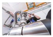
(Photograph: JPS \_Prüfstand Detail.JPG, Source: Jung Process Systems) Flexible connections enable all HYGHSPIN models to be tested on each test rig.
